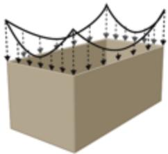
The greatest compression strength of CFB is within 1” of the edges created by two adjacent panels. The length of the dotted arrow is proportional to the load bearing ability at that point.
